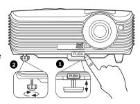
If the projector is not placed on a flat surface or the screen and the projector are not perpendicular to each other, the projected image becomes trapezoidal. To correct this situation, see "Correcting keystone" on page 26 for details.
